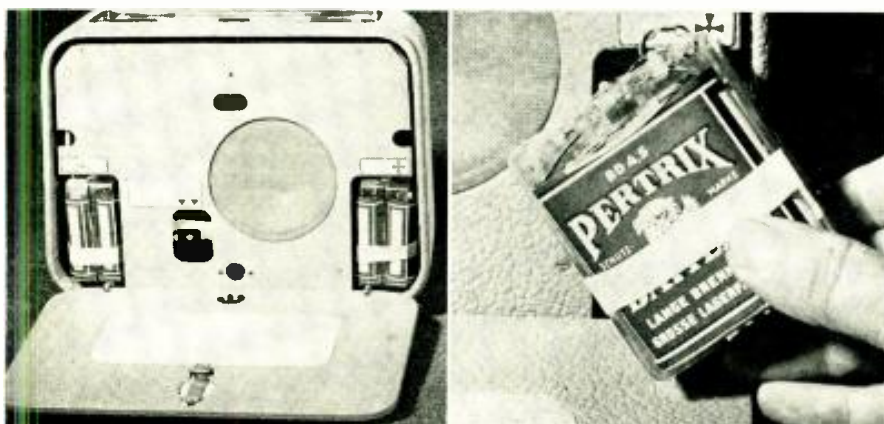
Back of case opened to show placement of batteries and speed shifting control. Batteries are standard 4 1/2 volt and fit in plastic holders which slide in the wells provided as shown. Back of recorder swings out to give access to batteries and speed shift.
