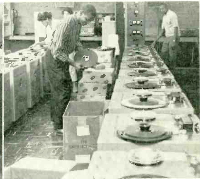
4 The console feeds the "slaves" and each tape is recorded individually with the signal from the master tape assuring top quality. Improvements in heads and amplifiers have made high speed duplication practical. Each machine turns out a single tape on each run. Tape supply is on large hubs. Below: enjoying the finished product at home.
