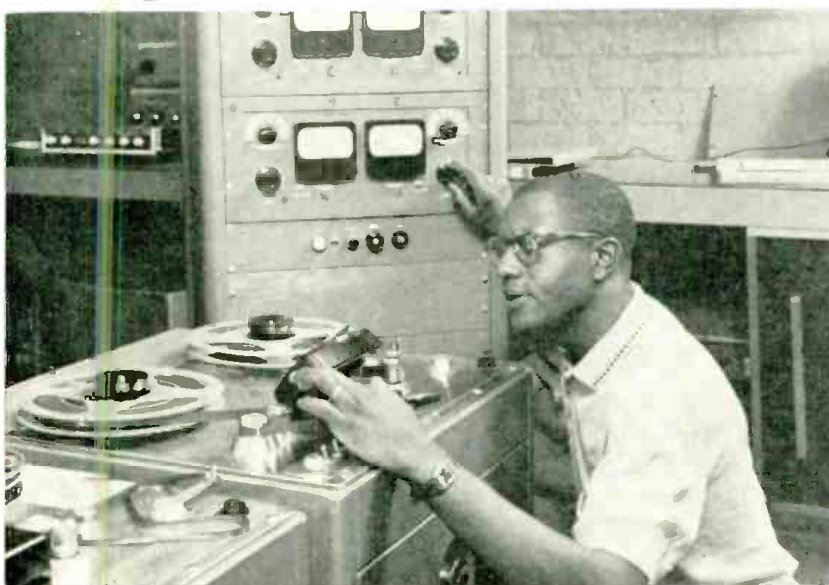
3 After the duplicating master has been made the tape is further checked out on the master console before beginning a production run. Now that four track tape is here, the operator must be sure that all four channels stay within a hairbreadth of each other. Tape speed is 120 ips.
