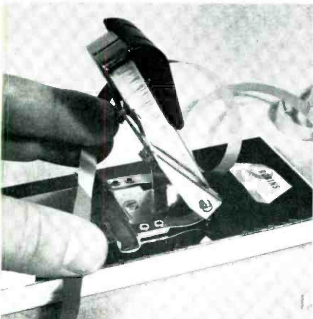
The Gibson Girl splicer gets its name from the shape of the finished splice. In addition to the channel to hold the tape, two blades are incorporated in the handle. One makes the diagonal cut through both ends of tape and the other trims the splice after the tape is applied.
